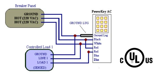
Wiring Diagram for PowerKey AC without an Auxiliary Device
