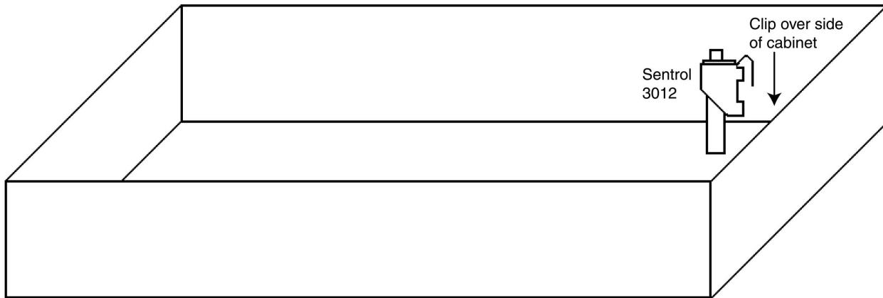
Figure 23: Installing a Tamper Switch
