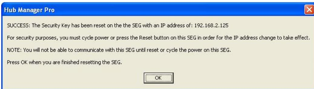
5. As a security measure, you must now go back to the SEG and either cycle power or press the reset button on the SEG. This sets the new security key into non-volatile memory. If you do not reset the SEG after the security key is reset you will not be able to communicate with the SEG.
