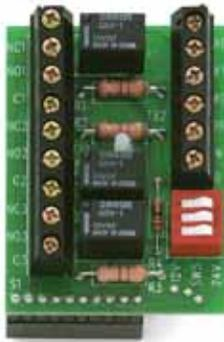
The 293 Relay Module provides three 1 amp Form C relays and the REX input via screw terminals for the 212i & 212w keypads. These keypads come from the factory with a harness that supplies a 50 mA source, but if relay outputs are required, the 293 is the perfect choice.
