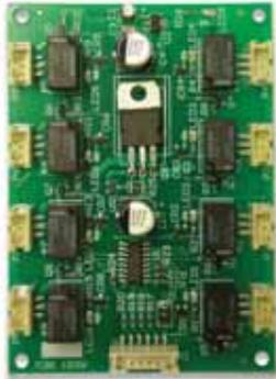
The 2000-8EX Output Expansion Module is for use with 2000 Series keypads and provides eight 1 amp Form C relay outputs. It wires to the keypad with 6-wire connection and is powered from the keypad. The module mounts to a double-gang electrical plate and can be installed up to 100' from the keypad.
