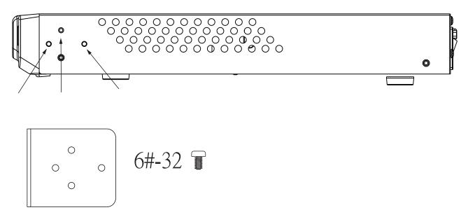
**3.** Secure the chassis to rack posts using two (2) M6 screws on each side.
