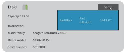
Note that disk verify function requires a volume to be temporarily disabled; namely, the video recording will be stopped before disk verify can be performed.
