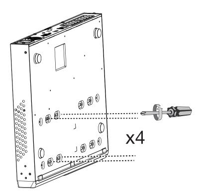
6. Secure the hard disks to the mounting positions in the chassis with its label side facing up and the connectors facing the inside of the chassis. The sample drawing below shows the positions.
