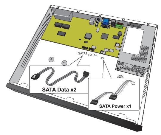
**4.** Connect the SATA power and SATA data cables to the hard drive.
