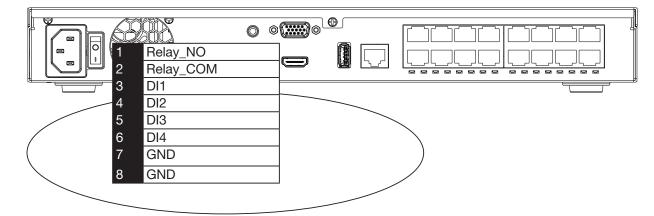
The GND are common ground for the DIs.
