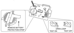
**STEP 10** Reset Trouble Indicator. Close transmitter cover and reset any trouble indicators on receiver caused by the open cover.
