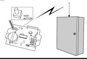
**STEP 12** *Wire Receiver.* Wire receiver obstacle output to obstacle input on operator. Refer to operator and receiver wiring instructions.
