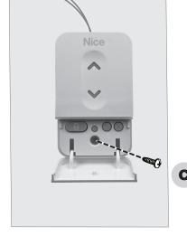
NOTE: The Wall Station is also sized to mount on a standard single gang box.
