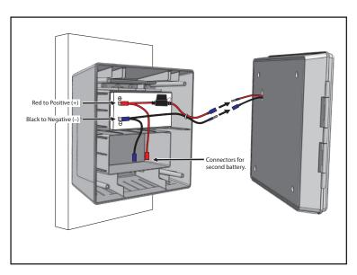
Tuck the excess battery leads into the battery box and reattach the CONTROL BOX to the BATTERY BOX.
