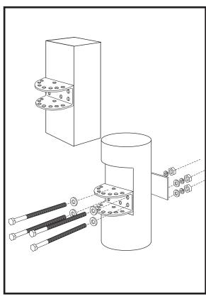
Close the gate and place your level against the horizontal cross member. Position the level so that the top should be in the center of the cross member and overlaps the post. Scribe a line across the cross member and post. You will use this line to help determine position of post and gate brackets.
