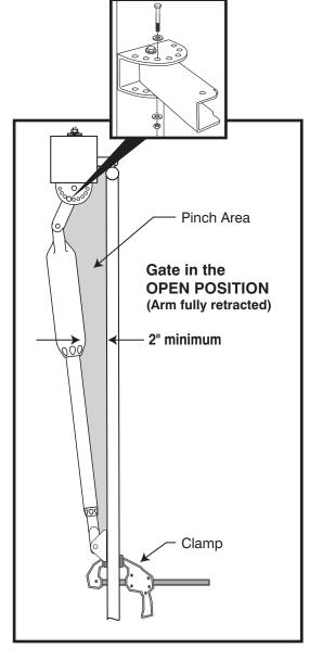
Remove the clevis pin from the front mount and while supporting the gate operator, swing the gate and gate operator to the closed position. With the gate and gate operator in the closed position check the clearance and be sure that the gate operator is not binding at the post pivot bracket.
