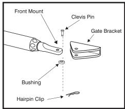
NOTE: Substitute a Pin Lock • [FM345] for the clevis pin on the front mount of the gate operator to prevent unauthorized removal of the operator from the gate.
