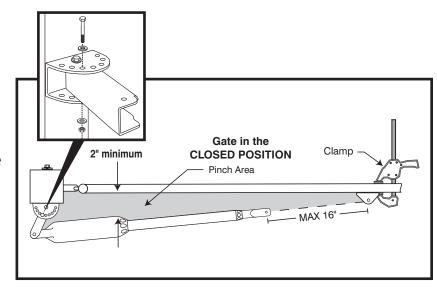
With the post pivot bracket in the optimum position for clearance and freedom of movement, replace the bolt in a post bracket adjustment hole and secure with 3/8" washer, and lock nut. Return the operator to the open position and reattach the gate bracket. Recheck the gate operator level and clearance in the open position. Adjustment of the gate bracket will be necessary if the post bracket was moved. After verifying clearance, make sure the gate bracket is clamped securely.
