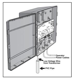
Strip 3/16" off the ends of the low voltage wire and twist tightly. Attach these ends to the 18 VAC or SOLAR terminals located on the POWER INPUTS terminal block. Be certain not to let the exposed wires touch each other!
