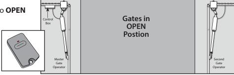
position, then press and hold the LEARN MAST LIMIT and/or the LEARN 2ND LIMIT button for 5 seconds. This will clear the memory for the closed limit position. Repeat Steps 1-6.
