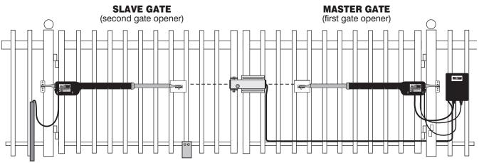
Lock and receiver must be level and aligned with opener.
