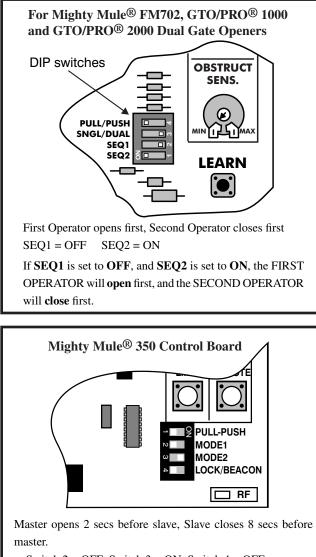
Switch 2 = OFF Switch 3 = ON Switch 4 = OFF
