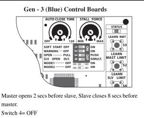
If **Switch 4** is set to **OFF**, the MASTER OPERATOR will **open** first, and the SLAVE OPERATOR will **close** first.
