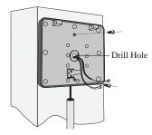
**Step 2:** Determine how the wires will enter the keypad (e.g., from the back through a hole drilled in the post; running the wire on the post surface). Drill a hole in the back of the keypad cover and pull the wire into the cover. Then mount the cover to the post using the screws provided. Run wire through PVC pipe from the ground to keypad and from the ground to the opener control board to protect it from lawn mowers or grazing animals.
