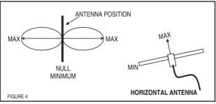
**NOTE:** The horizontal antenna can also be used to null out interfering signals. If a known source of interference (such as a military base or computer system) is known, the null minimum can be oriented so that it is towards the interference.
