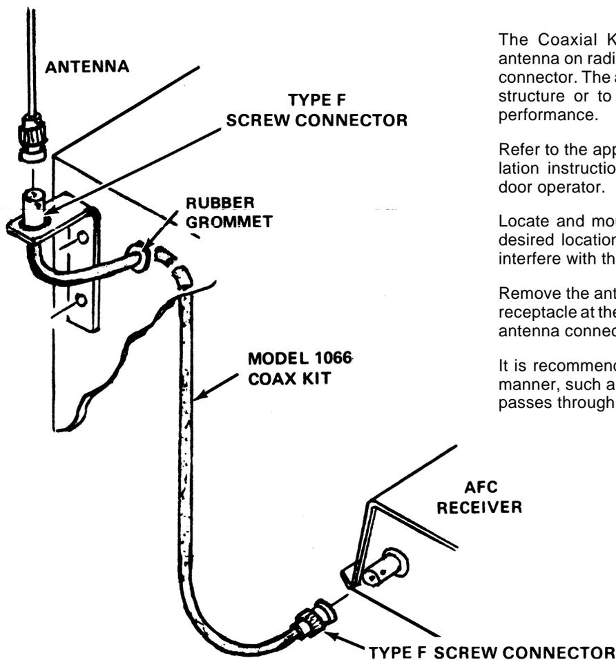
The Coaxial Kit permits the remote location of the antenna on radio receivers equipped with a type F screw connector. The antenna can be moved away from a metal structure or to an outside location for better receiver performance.
