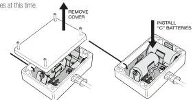
**Attention:** Consult the battery manufacturer's product datasheet for battery specifications (i.g., operating temperature range, battery Life cycle, etc). Utilizing product outside of the manufacturer's specifications may result in unexpected behavior and require special maintenance requirements. NSC recommends replacing the battery at least annually if using the product in an environment outside the battery manufacturer's specifications.
